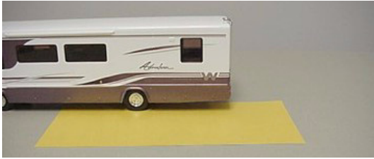
Weighing Left Rear 'Corner'
