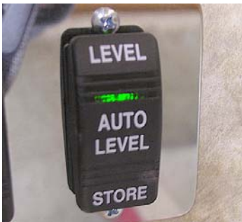
Auto Level Switch inside Entrance Door
