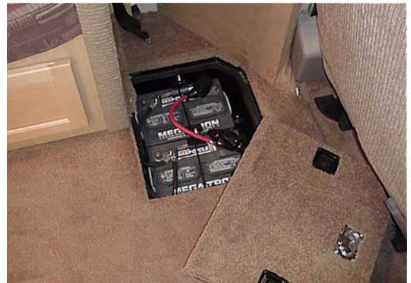
House Batteries in floor behind driver seat
