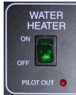
Gas Water Heater Switch (on Systems Monitor Panel)
