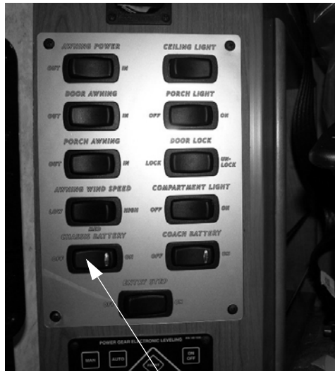
Chassis Battery Disconnect Switch (Located near entrance door) -Typical View
