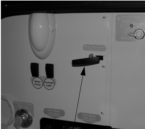
Water Tank Drain Valve (Located in water service center - pull to drain) -Typical View
