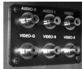
Audio Video Connection Plate -Typical View
