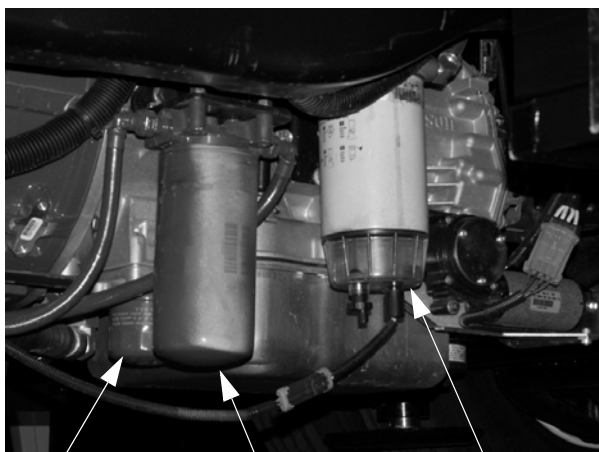
Transmission Fluid Filter (Typical) Engine Oil Filter (Typical) Diesel Fuel/Water Separator Filter (Typical)
