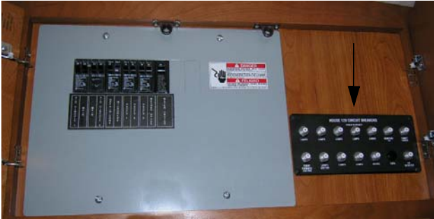
House 12-Volt Circuit Breaker Panel -Typical View
