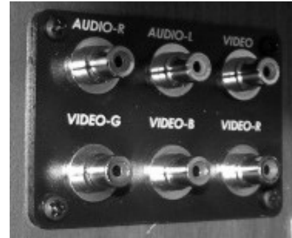
High Definition Audio Video Connection Plate (Located in cabinet near TV) -Typical View
