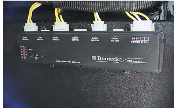
Awning Control Box (Located in exterior compartment)
