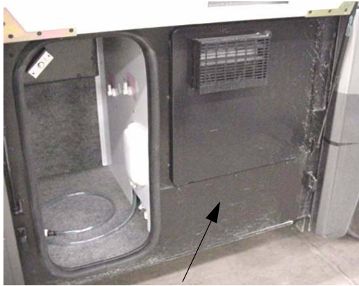
Water Pump Access Panel (Your model may or may not be equipped with an access panel) -Typical View
