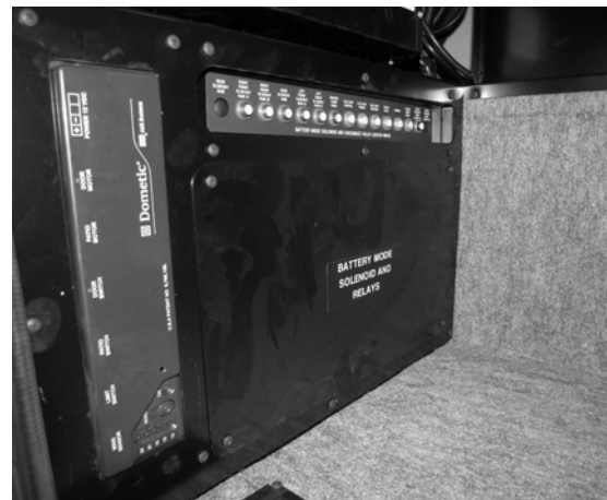
Auto Chassis 12V Circuit Breaker Panel (Located inside first compartment to the right of the entrance step) * Models 32H, 35P, and 37F -Typical View
