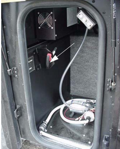
Water Tank Drain Valve - Model 38N shown (pull to drain) -Typical View
