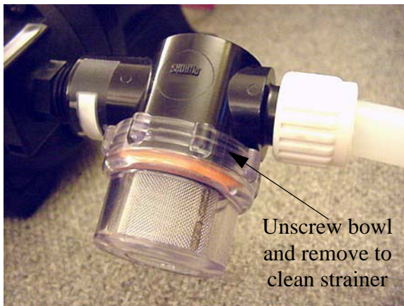
Water Pump Strainer -Typical View
