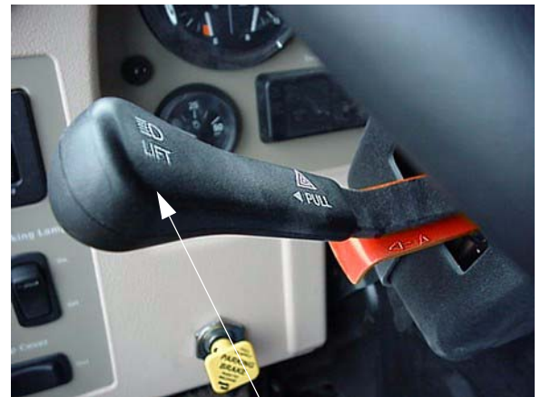
Turn Signals/Hi-Lo Beams (Typical View - your coach may differ depending on model)
