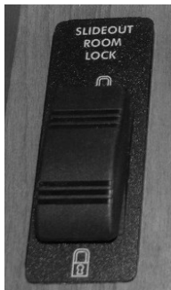
Slideout Room Travel Lock (Your model may be equipped with one or more types) -Typical View
