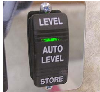
Auto Level Switch (Located inside entrance door -Typical View
