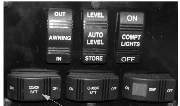
House/Coach Batt Disconnect Switch (Located near entrance door) -Typical View
