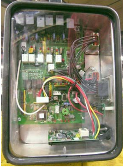
Hydraulic System Control Box (Located on pump beneath chassis near LH or RH front tire)
