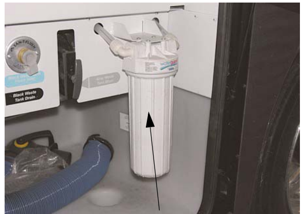
Full-Coach Water Filter System (Located in water service center) -Typical View
