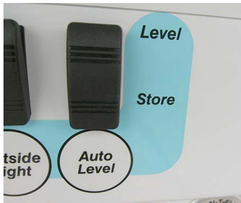
Auto Level Switch (Located in service center compartment) -Typical View
