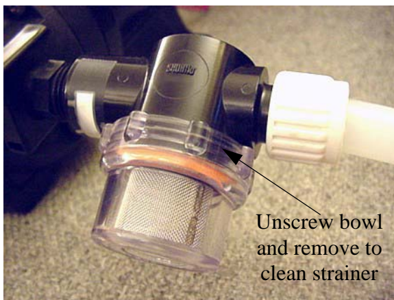
Water Pump Strainer -Typical View
