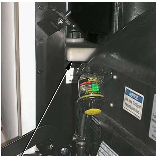
Power Steering Fluid Reservoir in recessed area at LH side of rear engine service compartment
