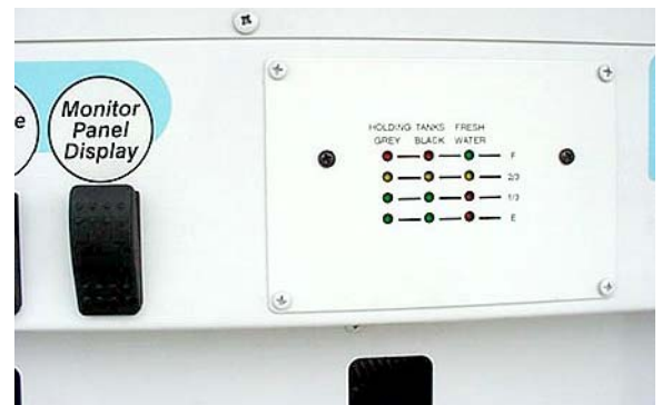
Water Center Tank Level Monitor -Typical View
