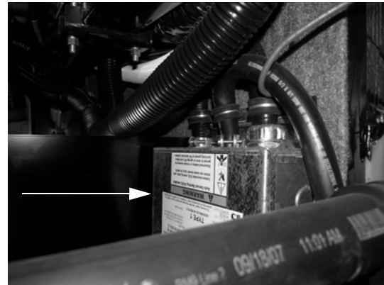
Automatic Power Transfer Box (Located inside or behind utility compartment) -Typical Installation
