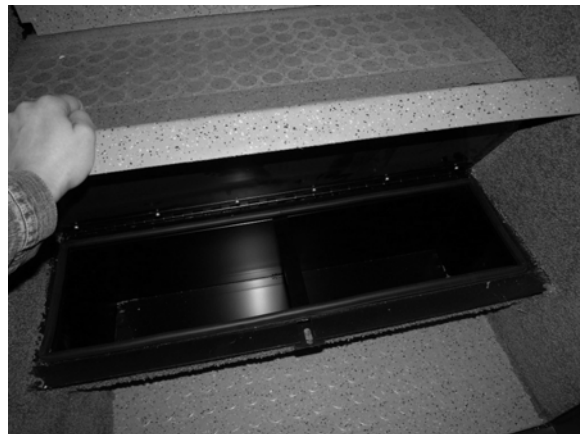
Entry Step Storage (Lift removable storage bin out to access hydraulic pump)
