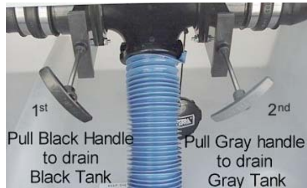
Holding Tank Valves (Typical)
