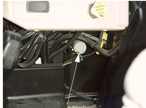
Diagnostic Plug (Located on steering column support plate beneath left side of dash) -Typical View
