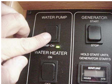
Water Pump Switch (Located on the monitor panel) -Typical View
