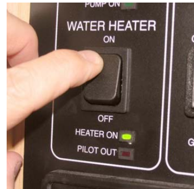
Gas Water Heater Switch (Located on monitor panel)
