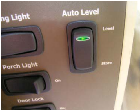
Auto Level Switch (Located inside entrance door) -Typical View
