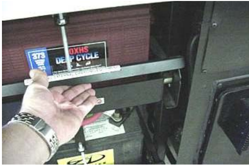
Lift Battery Tray Retainer Latches
