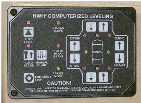
Leveling System Control Panel (Located near dash)
