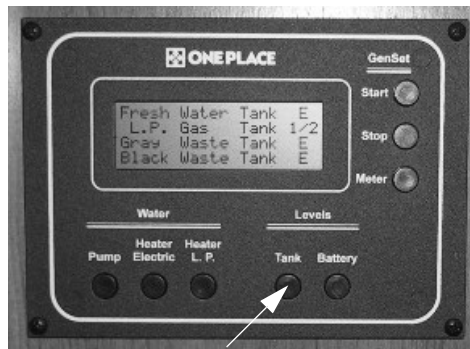
Tank Levels Switch
