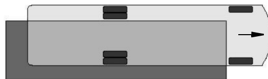
Weighing Right Rear Corner
