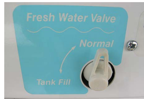
Fresh Water Valve in Normal use position (Located in water service center)
