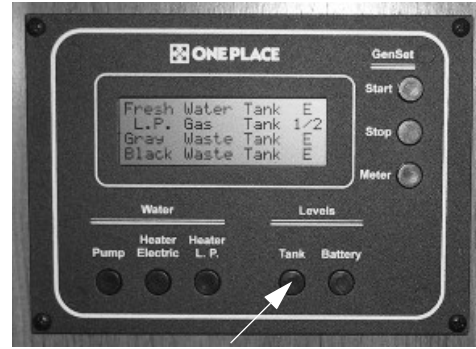
Tank Levels Switch
