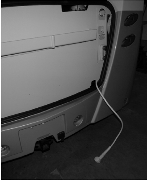
Using exterior shower to drain waterline
