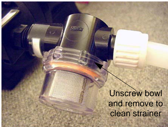
Water Pump Strainer -Typical View
