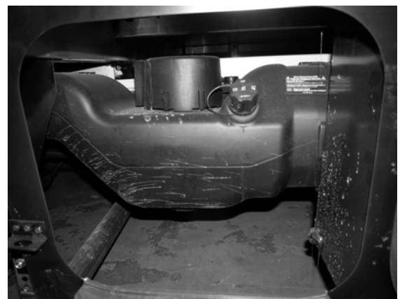
Diesel Exhaust Fluid Fill Tank (Located in passenger side compartment behind entrance door) -Typical View
