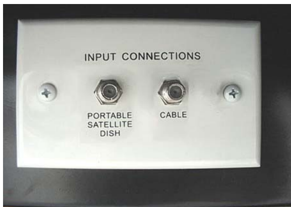
Cable TV and Satellite Dish Input Connections (Located in shoreline or utility compartment, depending on model)
