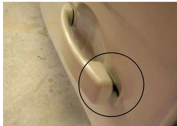
Door Unlatched (note gap)
