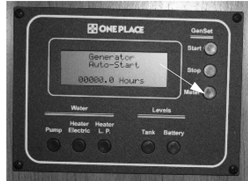
Generator Hourmeter Button -Typical View
