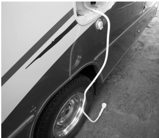
Using exterior shower to drain waterline (Typical View - appearance on your coach may differ)
