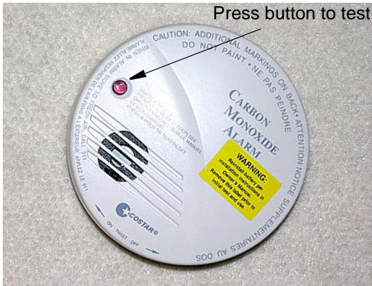
Carbon Monoxide Alarm
