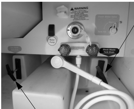
2nd - Pull Gray Waste Tank Drain valve to drain Gray Water (sink/shower) tank – then close.
