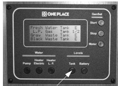
Tank Levels Switch
