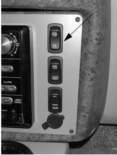
Defrost Fan Switch -Typical View
