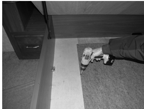
Removable Panel (if equipped) (Located underneath bed) * Lift bed board to access -Typical View
