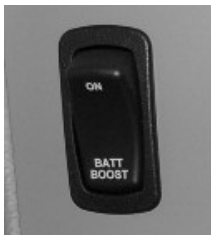
Battery Boost Switch (Located on dash)
