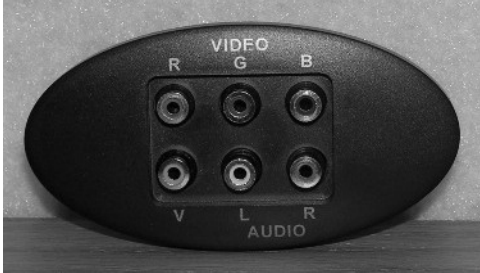
Audio Video Connection Plate -Typical View
