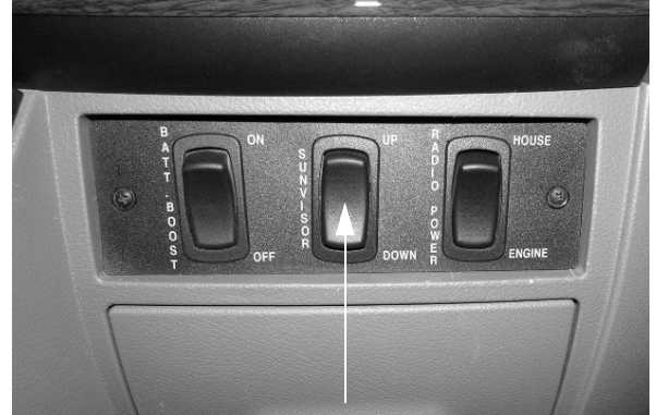
Power Sunvisor Switch (Located beneath cab radio) -Typical View
