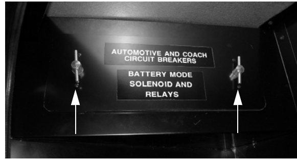
Chassis and House 12V Breaker Panel (Located in passenger side compartment) -Turn both latches to remove cover
