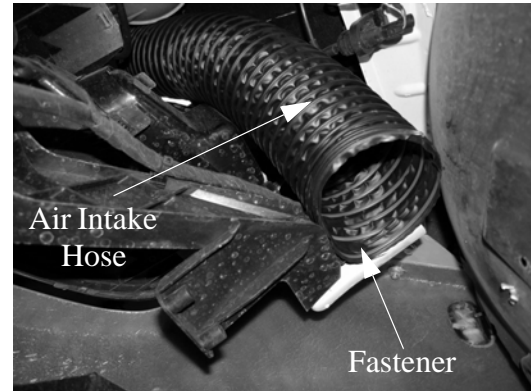
Air Intake Hose/Fastener (View shown from beneath the front end of coach)
