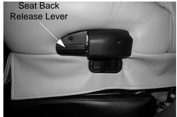
Seat Back Release Lever (Located on the side of cab seats)
