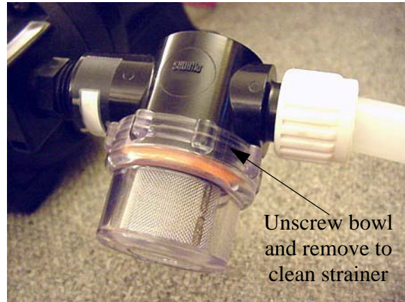
Water Pump Strainer -Typical View
