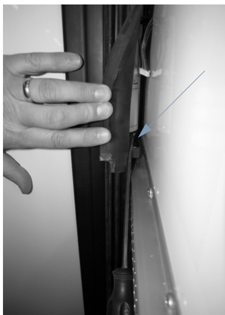
Slideout Motor (Located behind slideout wipe seal)
