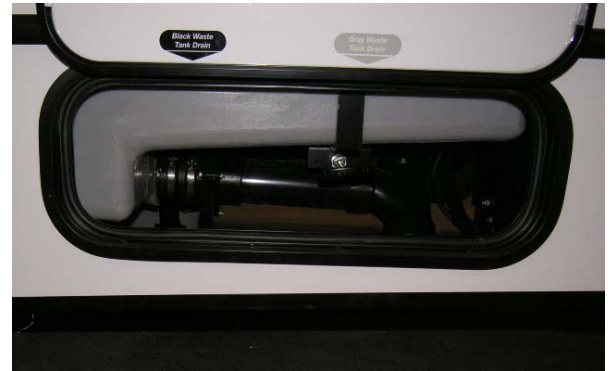
Holding Tank Dump Valves (Located in mid-driver side access compartment) -Typical View
