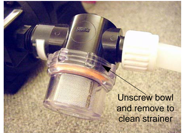
Water Pump Strainer -Typical View
