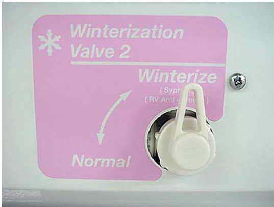
Winterization Valve 2 (Located near water pump - second compartment on driver side of coach)
