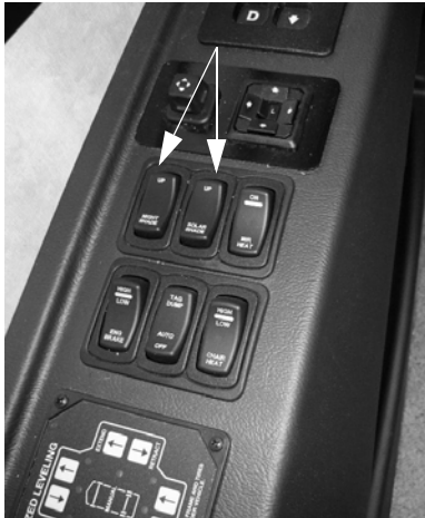
12-Volt Front Drop-Down Solar/Night Shade Switches (Located on driver side trim panel) -Typical View
