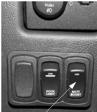
Battery Boost Switch (Located on dash)
