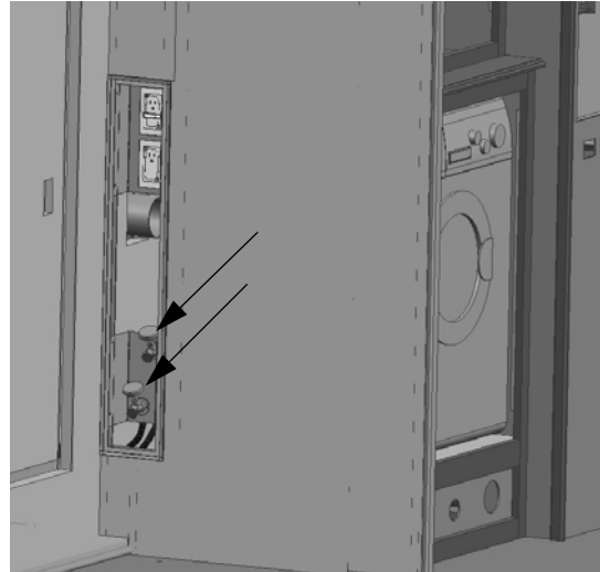
Water Supply Faucets (Located along left-hand side of Stackable Washer/Dryer cabinet - remove panel to access)
