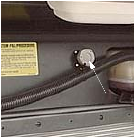
Diagnostic plug on rear engine compartment shroud -Typical View
