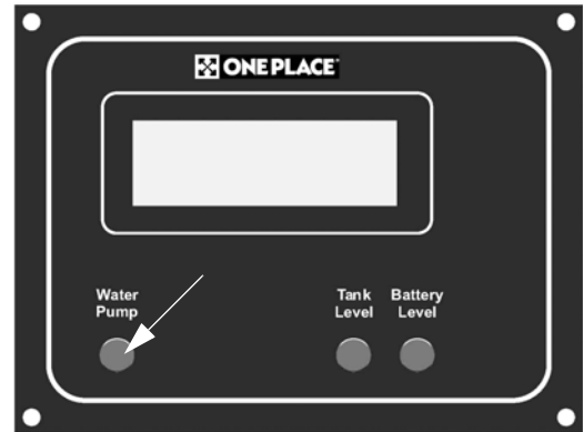
Water Pump Switch
