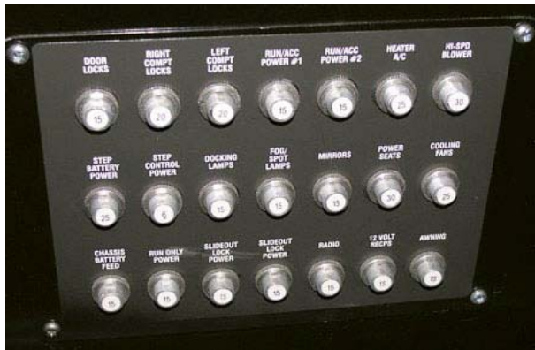
Automotive Circuit Breakers (push to reset) Breakers are labeled for components equipped
