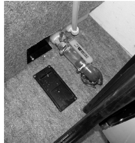
Water Tank Drain Valve (Located in first passenger side compartment) -Typical View
