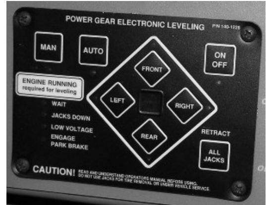
Leveling System Control Panel
