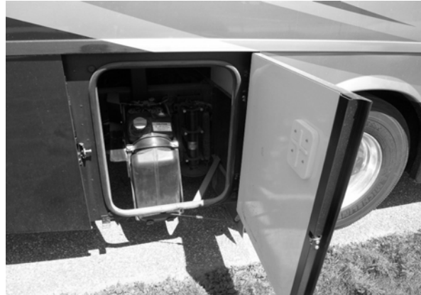
Diesel Exhaust Fluid Fill Tank (Located in passenger or driver side compartment behind rear wheel, depending on model) -Typical View
