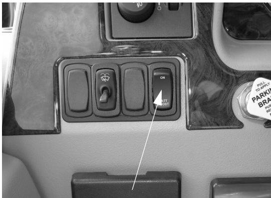
Battery Boost Switch (Located on dash)
