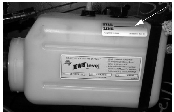
Hydraulic Oil Reservoir (Located underneath front entry step) -Typical View
