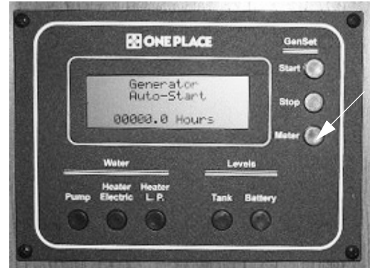
Generator Hourmeter Button -Typical View
