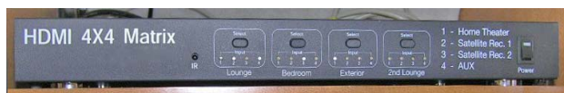
HDMI Video Selection System (Located in front passenger overhead cabinet) - Model 42E only
