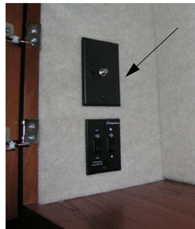
TV Signal Amplifier Power Switch (Located in overhead cabinet above entry door)
