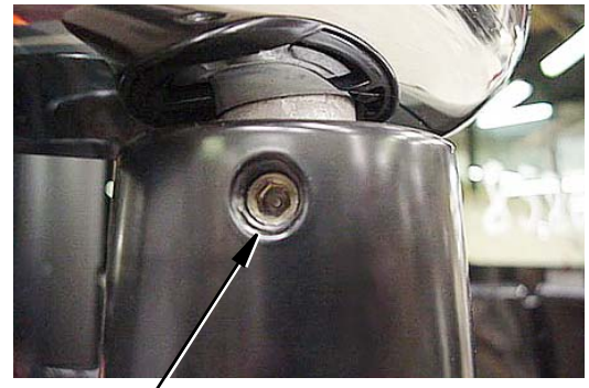
Allen Head Set Screw* (Torque screw to 75-100 in./lbs.)
