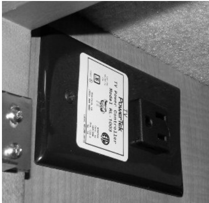
Front TV Ignition Switch Interlock -Typical View
