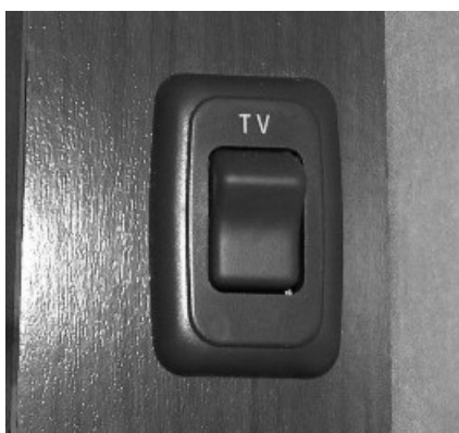
12-Volt Master Power Switch (Located on end of galley cabinet) -Typical View
