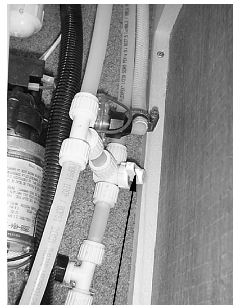
Waterline Drain Valve (Typical)
