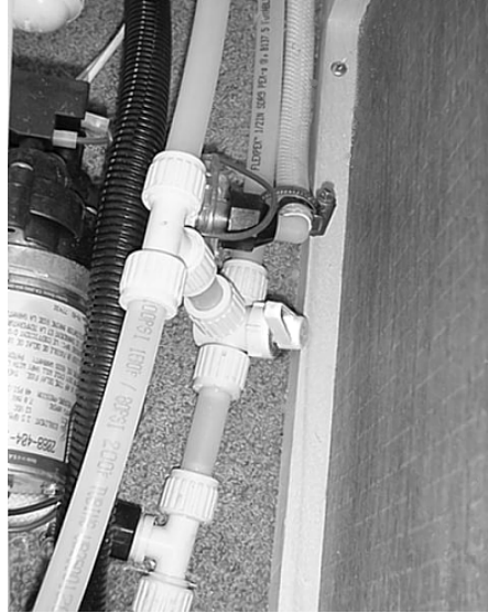
Waterline Drain Valve (Located behind access panel in rear storage compartment) -Typical View
