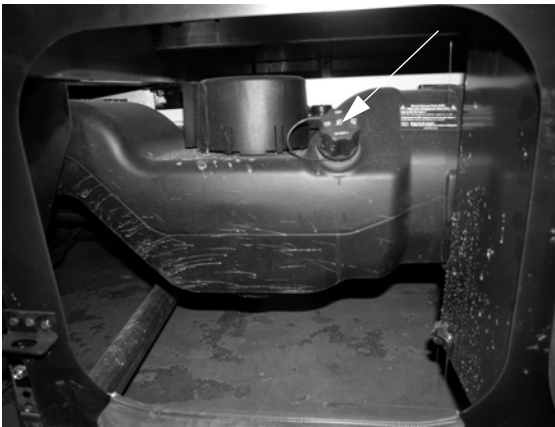
Diesel Exhaust Fluid Fill (Located in passenger side compartment behind entrance door) -Typical installation shown
