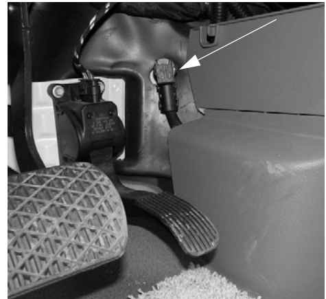
Chassis Battery Connector (Located to the right of the accelerator pedal)
