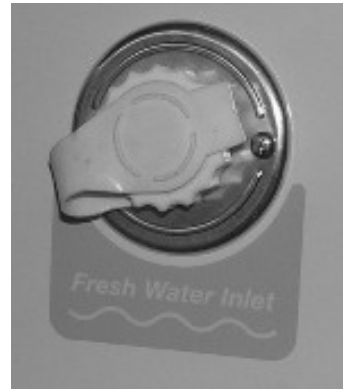
Fresh (City) Water Connection (Fresh Water Inlet)
