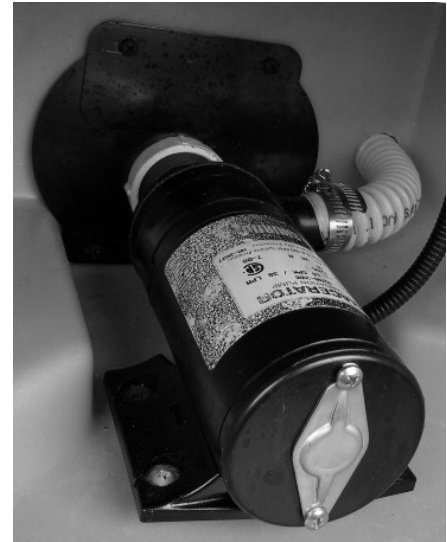
Waste Pump (Located behind removable panel in water service center) -Typical View
