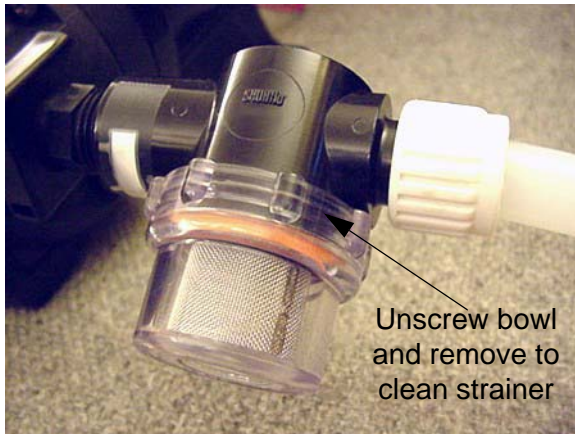
Water Pump Strainer -Typical View
