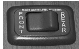
Black Waste Tank Selector Switch (Located near monitor panel) -Typical View
