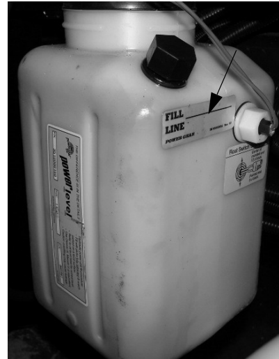
Hydraulic Oil Reservoir -Typical View
