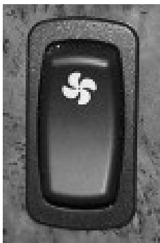
Defrost Fan Switch (Located on dash)
