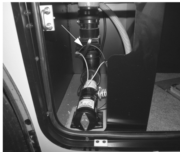
Black Waste Tank Drain Valve #1 (Front) (Located in passenger side compartment ahead of rear axle) -Typical View
