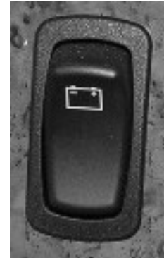
Battery Boost Switch (Located on dash)
