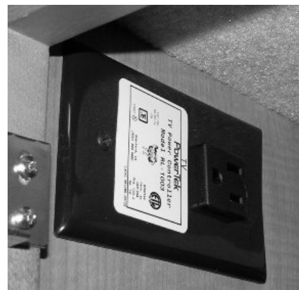
Front TV Ignition Switch Interlock -Typical View
