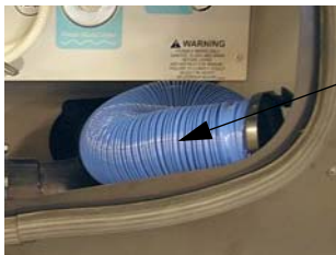
Sewage Drain Hose -Typical View
