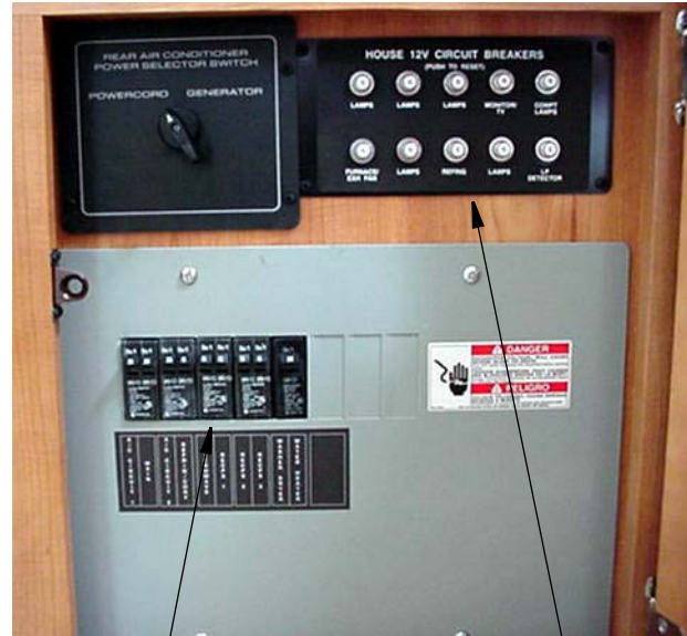
120-Volt House Circuit Breakers 12-Volt House Circuit Breakers Power Center (32', 35', and 36' models) -Typical View
