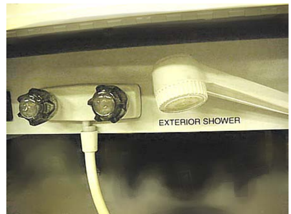
Exterior Shower/Wash Station -Typical View
