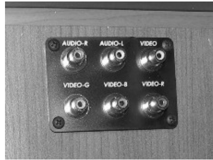
AV Connections (Located in galley or bedroom overhead cabinet - if equipped) -Typical installation shown
