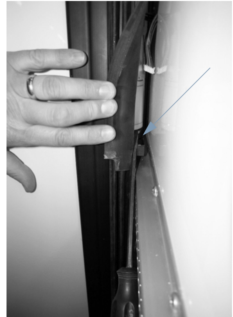
Slideout Motor (Located behind slideout wipe seal)
