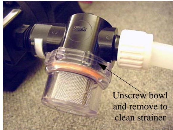
Water Pump Strainer -Typical View
