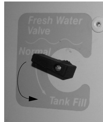
Fresh Water Valve (Located in water service center)
