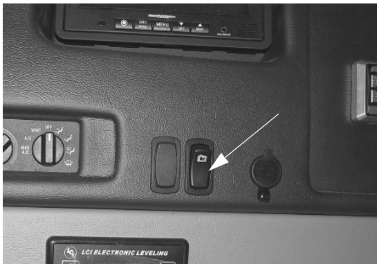
Radio Power Switch (Located on dash) -Typical View
