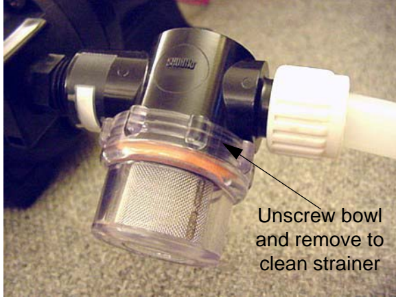
Water Pump Strainer -Typical View
