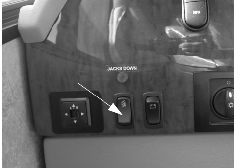
Mirror Heat Switch (Located on dash) -Typical View
