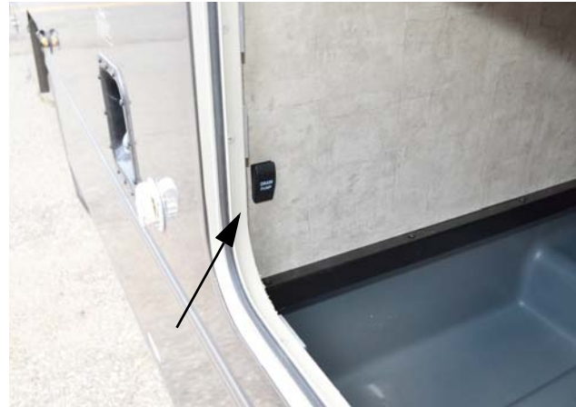
Waste Pump Switch (Located in driver side compartment) -Typical View
