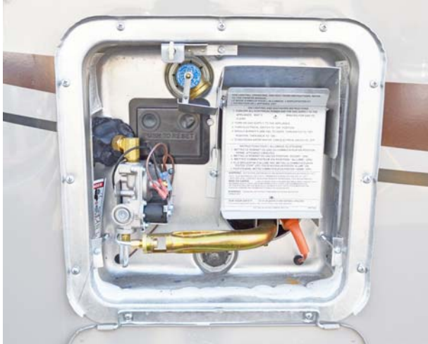
Water Heater Exterior Service Access
