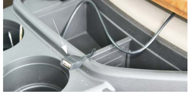
USB Cable (Located in the beverage tray) -Typical Installation
