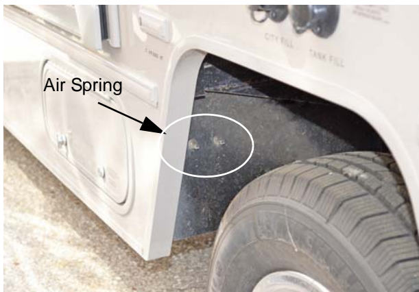
Rear Air Spring Valves (Located inside left rear wheel well -Typical View
