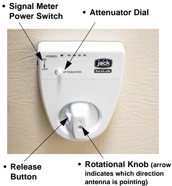
Digital Antenna Signal Meter (Located on ceiling)
