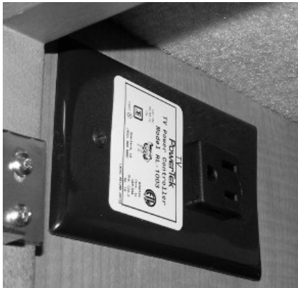
Front TV Ignition Switch Interlock -Typical View
