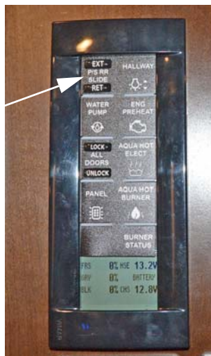
Rear Slideout Switch (Your coach may have one or more of these switches depending on model, options, and available equipment) -Typical View
