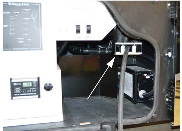
Power Cord Reel (Located in a driver side compartment) -Typical View
