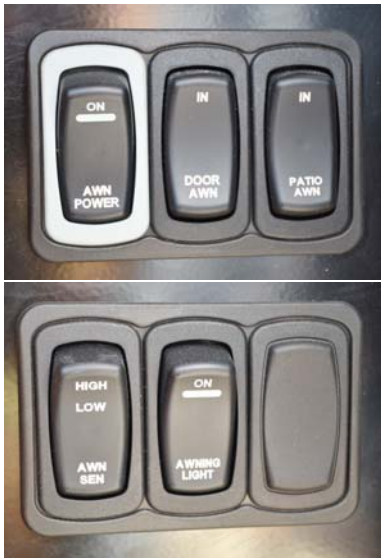
Power Awning Control Switches (Located near the entrance door) -Typical View
