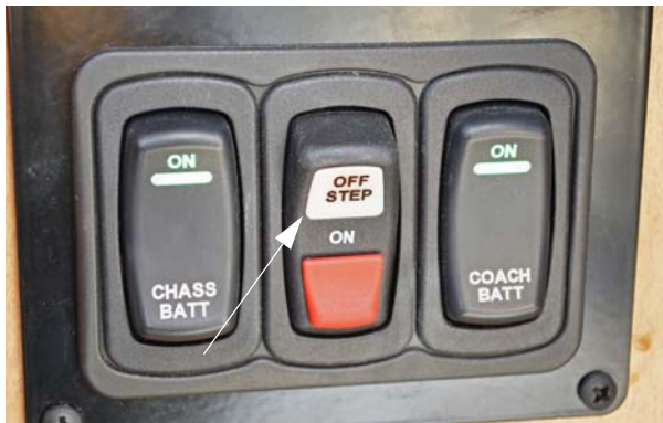
Entry Step Switch (Located near entrance door) -Typical View
