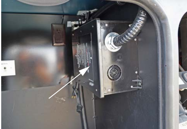
Automatic Power Transfer Box (Located inside or behind utility compartment) -Typical installation shown
