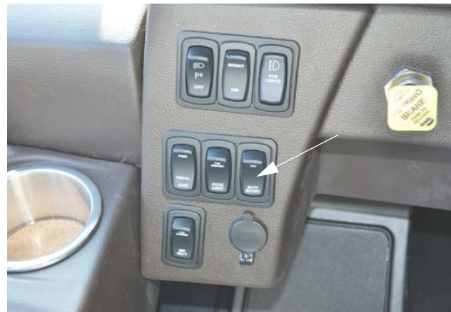
Battery Boost Switch (Located on dash)
