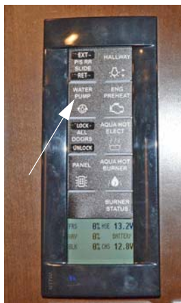
Water Pump Switch (Located on OnePlace cabinet and exterior water service center)
