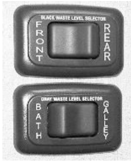
Black and Gray Waste Level Selector Switches (Located near monitor panel)
