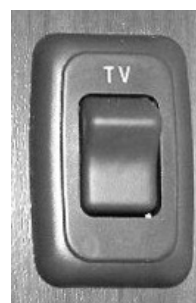
Bedroom TV 12-Volt Master Power Switch (Located on cabinet or wall near TV) -Typical installation shown
