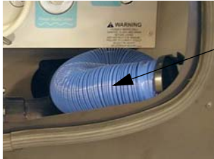
Sewage Drain Hose -Typical View
