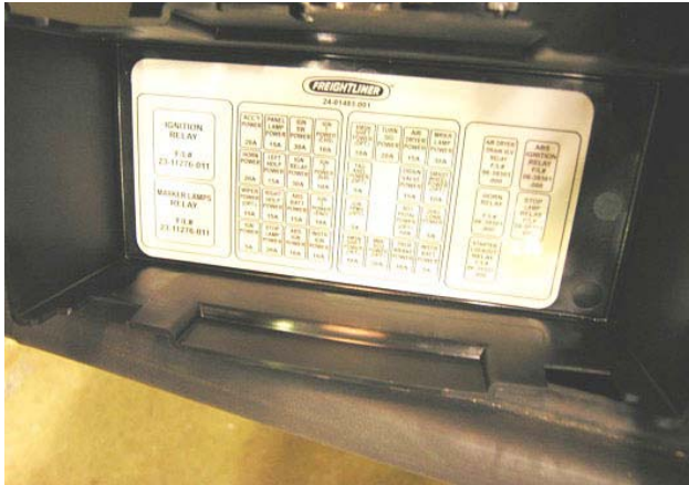
Fuse Diagram (inside of cover)
