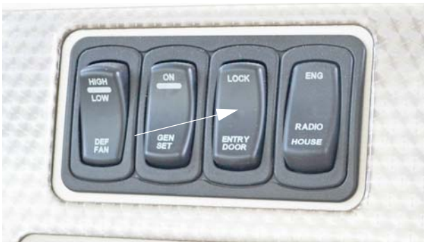
Power Door Locks - Entry Door (Located on dash) -Typical View
