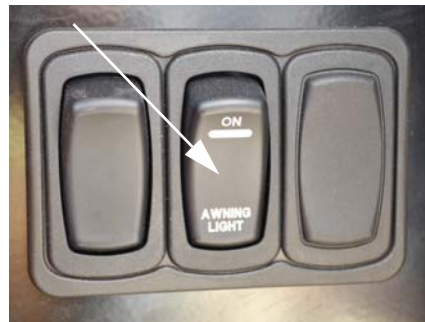
Awning Light Switches (Located near entrance door) -Typical View
