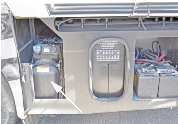
Diesel Exhaust Fluid Fill Tank *with Rear Radiator (Located in driver side compartment behind the rear wheel) -Typical View
