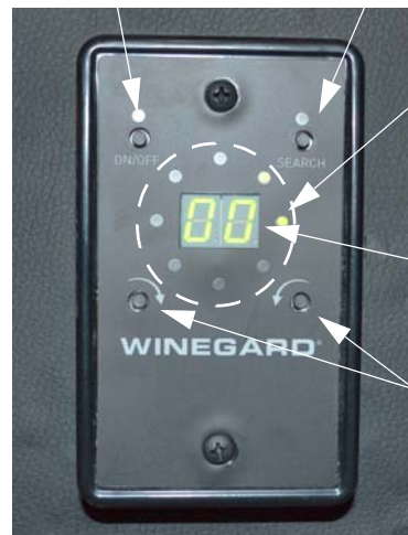
Digital Antenna Power Switch (Located inside entrance door overhead cabinet) -Typical View
