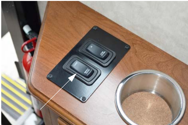
Power Door Locks - Entry Door (Located on passenger side trim panel) -Typical View
