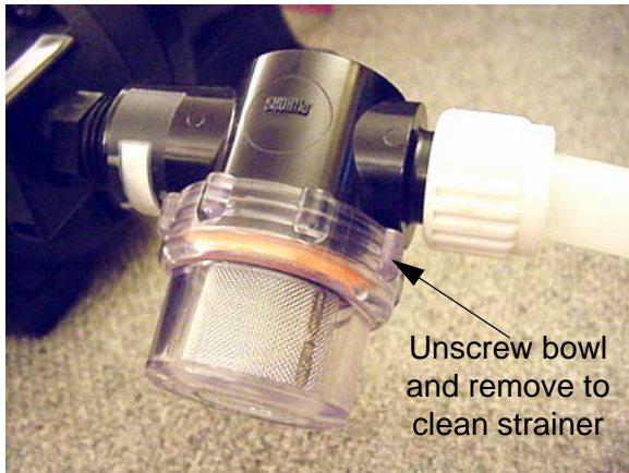
Water Pump Strainer -Typical View
