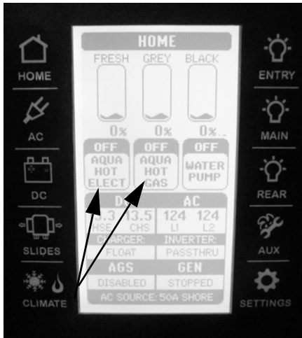
Hydronic Heating System Interior Control Switches “Home” Screen -Typical View
