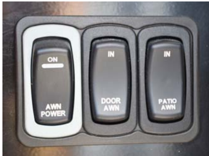
Awning Control Switches (Located near entrance door) -Typical View
