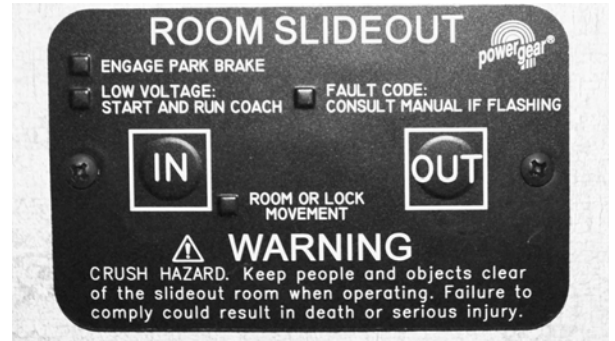
Slideout Switches (Located above entrance door) -Typical View
