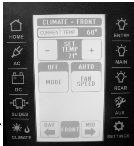
Thermostat “Climate” Screen (Located on Multiplex Monitor Panel)
