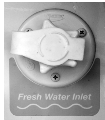
Fresh (City) Water Connection “Fresh Water Inlet” (Located in the water service center) -Typical View
