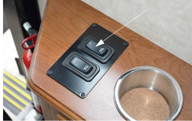
Step Cover Switch (Located on passenger side armrest) -Typical View
