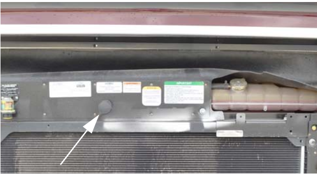
Diagnostic Plug *with Rear Radiator (Located on rear engine compartment shroud) -Typical View
