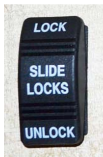
Slideout Room Travel Locks (Located above entrance door) -Typical View
