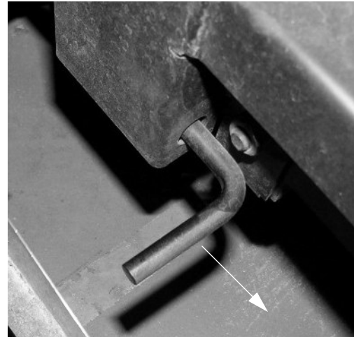
Release Lever (Located underneath the passenger side front hood)
