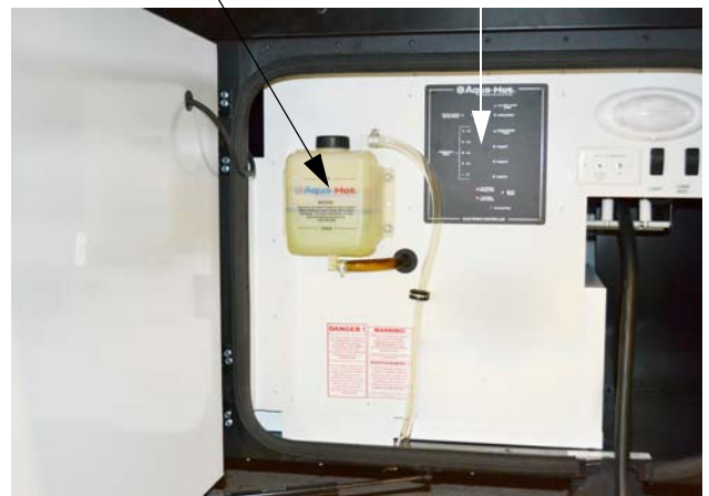
Hydronic Heating System (Located in driver side compartment) -Typical View
