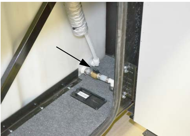
Water Tank Drain Valve (Located in first passenger side compartment) -Typical installation shown
