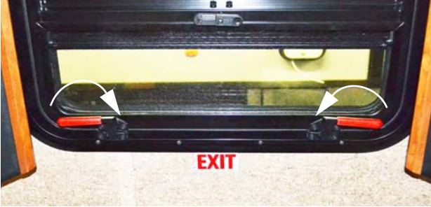
Escape Window (Lift both red safety latch handles UP and push window OUT) -Typical View
