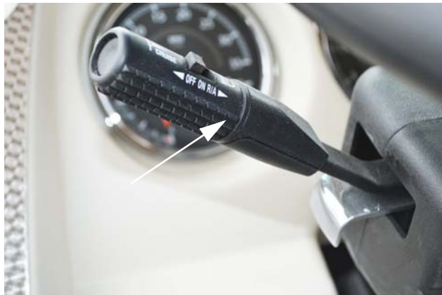
Turn Signals/High-Low Beams (Typical View - your coach may differ depending on model)
