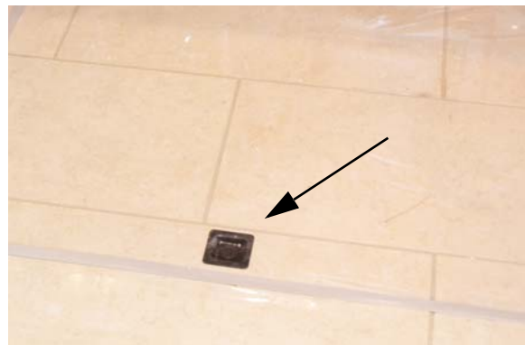
Engine Cover Latch -Typical View
