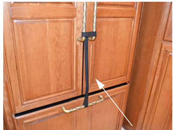
Refrigerator/Freezer Travel Latch (locked position)
