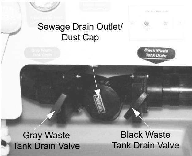
Holding Tank Drain Valves (Located in water service center) -Typical View Black and Gray Waste Tank Drain Valve positions may be reversed, depending on floorplan and tank location.
