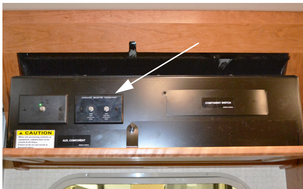
Interior Connection for Satellite Dish -Typical View
