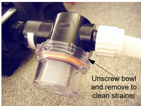
Water Pump Strainer -Typical View
