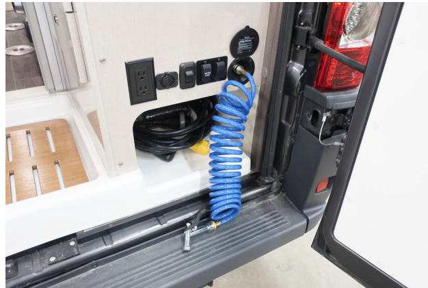
Exterior Shower/Wash Station (located behind rear passenger side door) *Model 59KL shown
