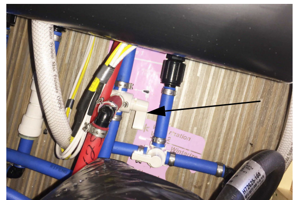
Winterization Valve 1 (Water Heater Bypass Valve) (See “Water System Drain Valve Locations” chart at the end of this section for location on your model) *Model 59KL shown
