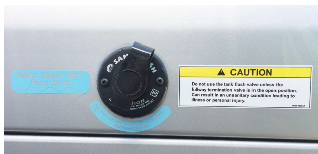
Black Waste Tank Flush Inlet (Located on left sidewall)
