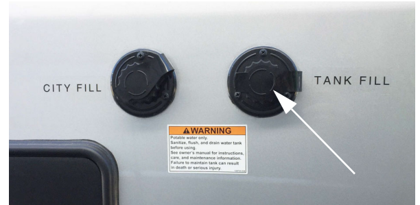
Tank Fill Inlet (Located on the left or right sidewall, depending on model) -Typical View
