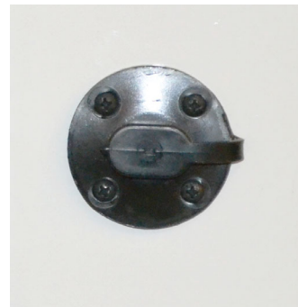
Single Solar Port (Located on an exterior sidewall or inside an exterior compartment, depending on model)
