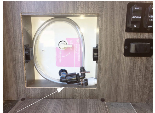
• Antifreeze Siphon Tube Antifreeze Siphon Tube/Winterization Port (See “Water System Drain Valve Locations” chart at the end of this section for location on your model) *Model 59GL shown
