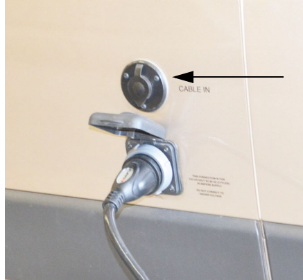
Cable TV Input Connection (Located on the left sidewall) *Model 59GL shown
