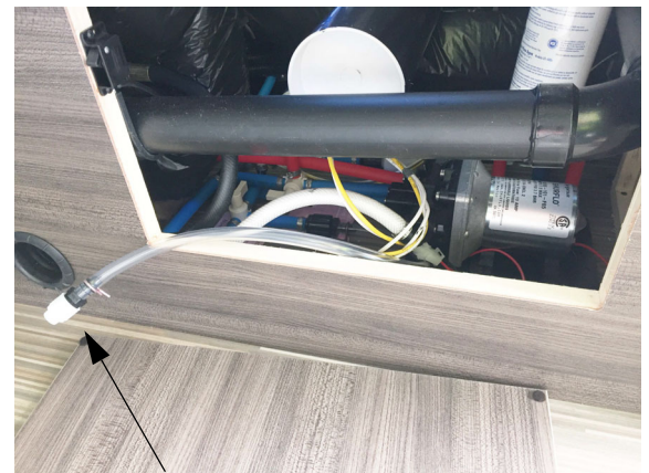
• Antifreeze Siphon Tube Antifreeze Siphon Tube/Winterization Port (See “Water System Drain Valve Locations” chart at the end of this section for location on your model) *Model 59KL shown
