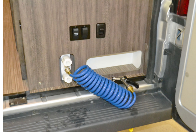
Exterior Shower/Wash Station (located behind rear passenger side door) *Model 59GL shown
