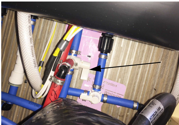
Winterization Valve 1 (Water Heater Bypass Valve) (See “Water System Drain Valve Locations” chart at the end of this section for location on your model) *Model 59KL shown
