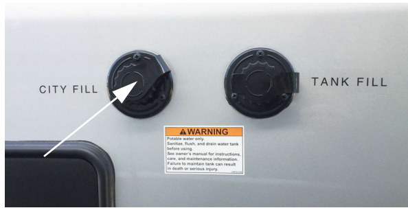
City Fill Inlet (Located on the left or right sidewall, depending on model) -Typical View
