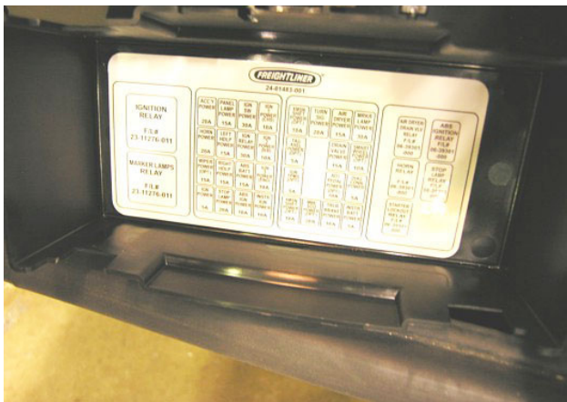
Fuse Diagram (inside of cover)
