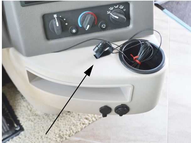
Bluetooth Microphone (Located near dash radio)
