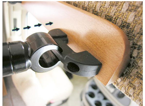
Attaching Bunk Ladder
