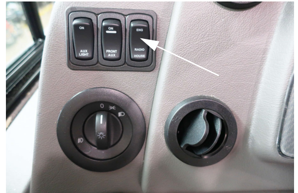
Radio Power Switch (Located on dash)
