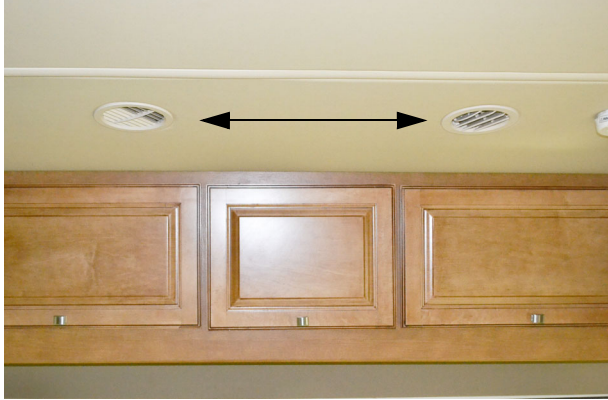
Supply/Return Air Vents (Located throughout the ceiling of the motorhome) -Typical View
