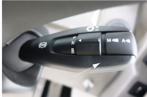
Exhaust Brake Switch (Located on driver’s steering column on the right hand stalk switch)
