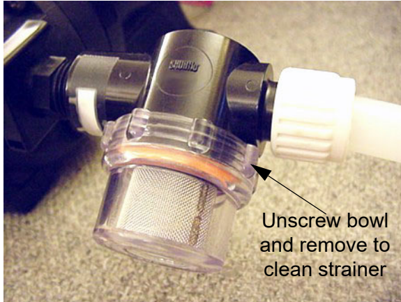
Water Pump Strainer -Typical View
