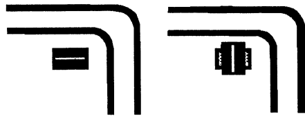
CLOSE OPEN Refrigerator Access Door Latches
