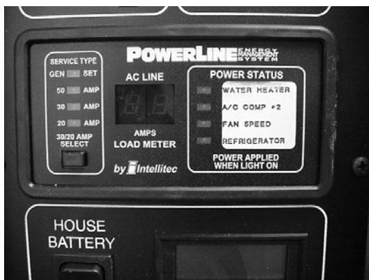
EMS Display on OnePlace Monitor Panel
