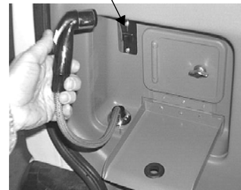
Water Pump Switch
