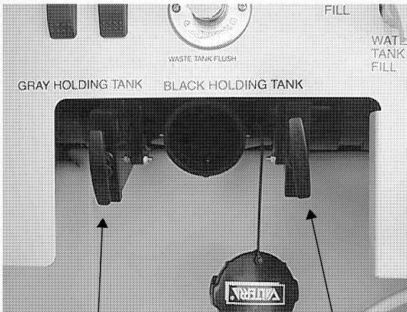
Pull last to drain gray tank Pull first to drain black tank
