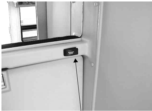
Shower Drain Pump Switch
