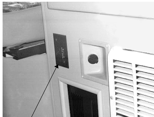
Water Heater Power Switch
