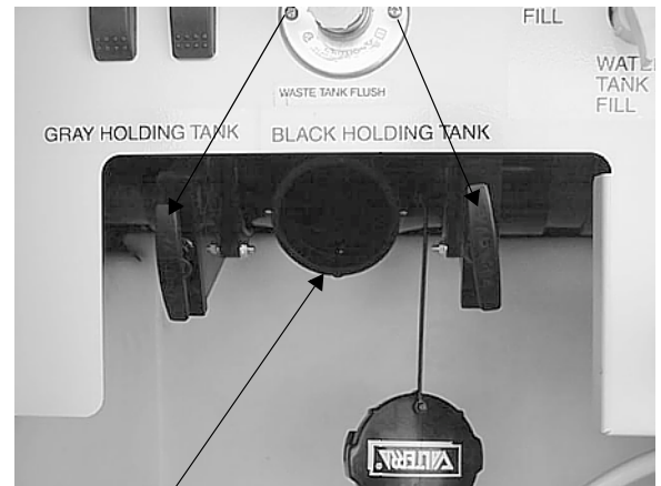
Sewage Dump Hose Outlet
