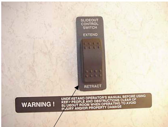
Bedroom Slideout Switch
