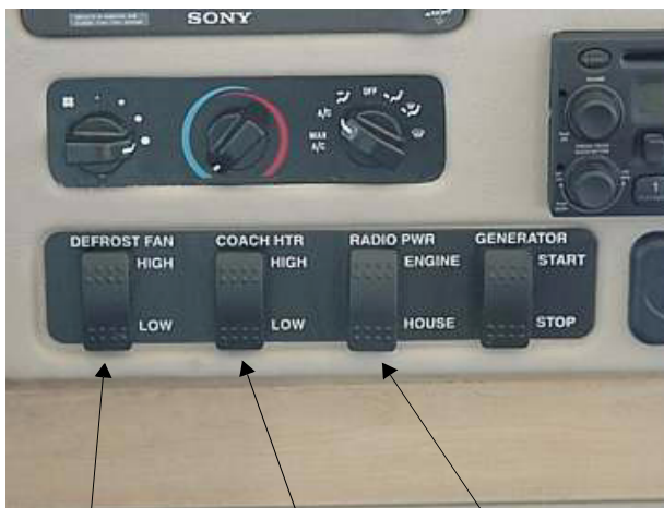
Windshield Defrost Fans Rear Coach Heater Switch Radio Power Switch
