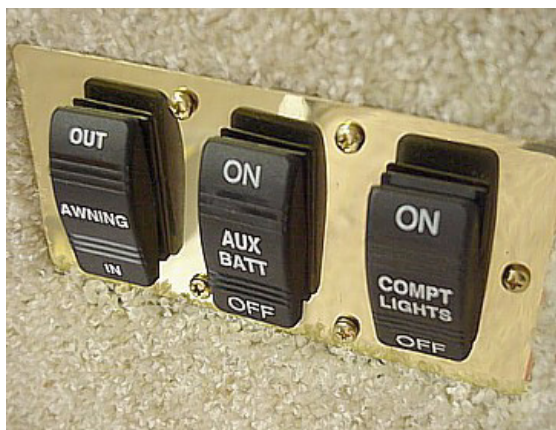
Aux. Batt. Disconnect Switch in Entrance Stepwell
