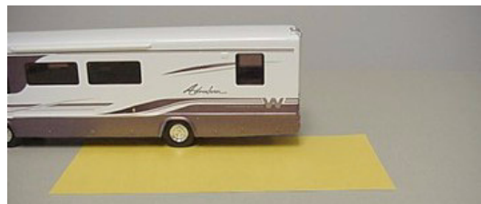
Weighing Left Rear ‘Corner’
