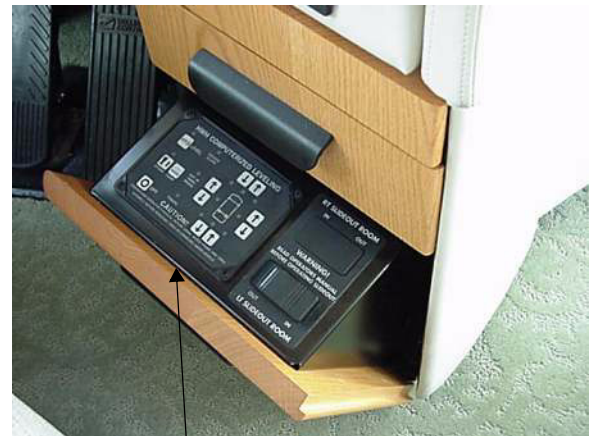
Automatic Leveling System Control Panel
