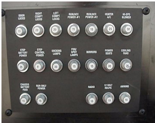
Automotive 12-Volt Breaker Panel
