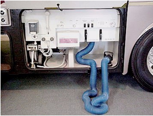
Black Tank Flush Inlet
