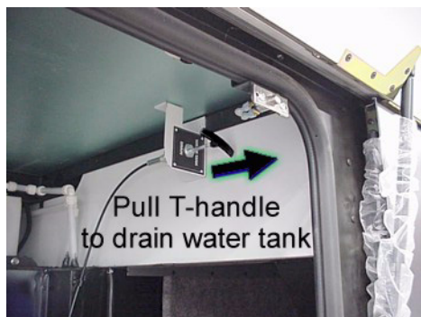
Water Tank Drain
