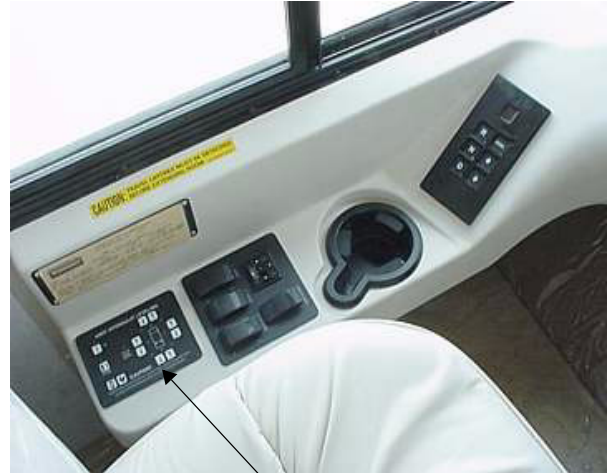
Leveling System Control Panel
