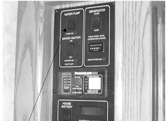
Water Pump Switch
