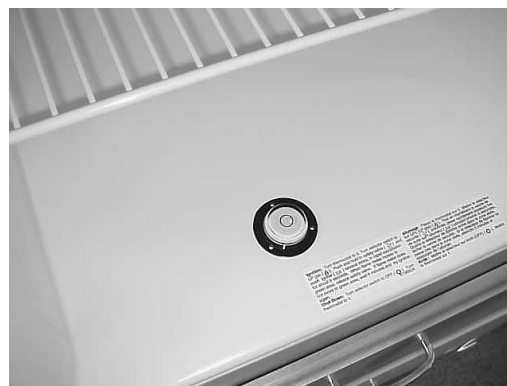
Place bubble level in bottom of refrigerator
