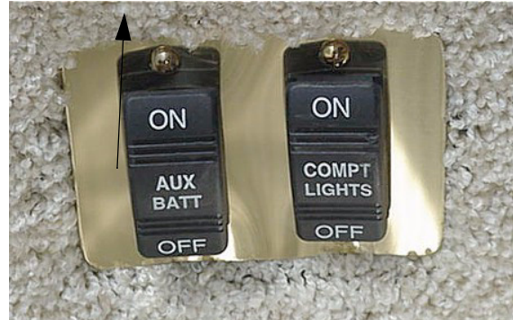
Aux Battery Switch (By Entrance Door)
