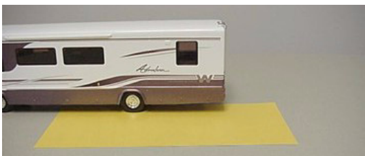
Weighing Left Rear 'Corner'
