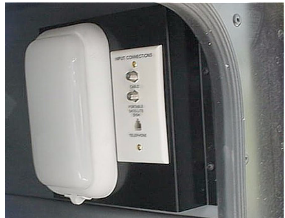
Exterior Connection for Satellite Dishes and Cable TV (In Utility Compartment)
