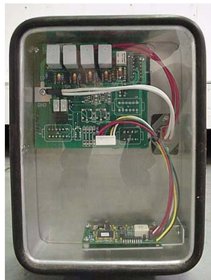
Hydraulic System Control Box on pump underside of coach near front tire
