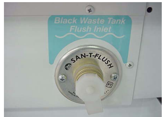
Water Tank Flush Inlet (typical)
