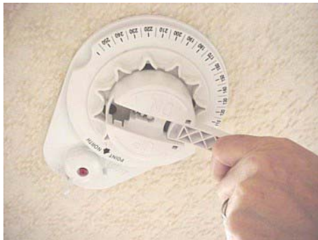
Digital Satellite Dish Control located on ceiling
