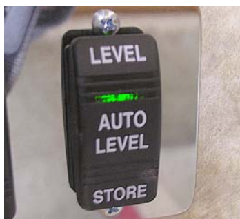
Auto Level Switch inside Entrance Door
