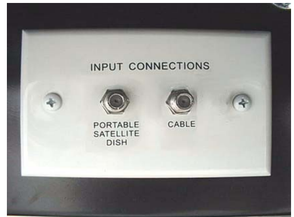
Exterior Connection for Satellite Dish and Cable TV (in Water Center or Utility Compartment)
