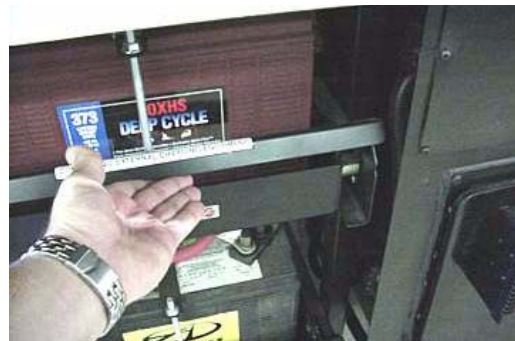
Lift Battery Tray Retainer Latches
