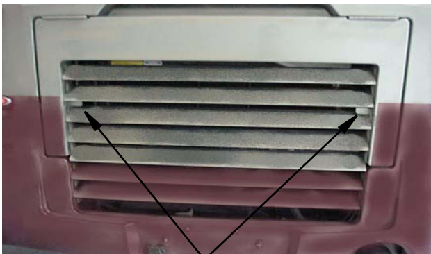
Lift latches and swing grille upward
