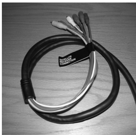
High Definition Accessory Connection Cables (Located in cabinet near TV)
