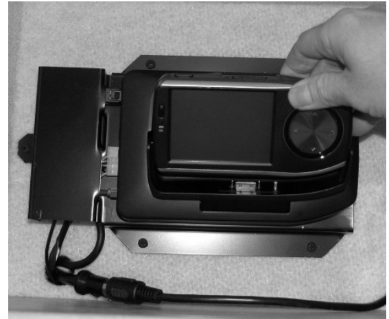
Portable GPS Navigation Docking Station (Located inside Driver's Side Overhead Compartment)
