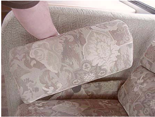
Remove armrest by pulling upward
