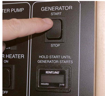
Generator Switch and Hourmeter on Monitor Panel
