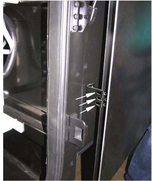
Remove 3 screws from front edge of condenser grille panel in locations shown.
