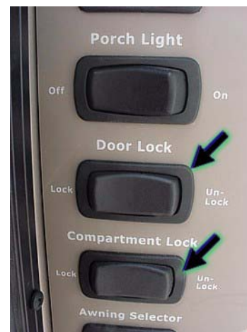
Power Door Locks on entry switch panel
