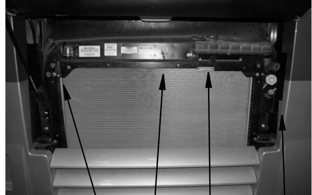
Air Filter Restriction Indicator Engine Diagnostic Connector Engine Coolant Reservoir Engine Oil and Transmission Fluid
