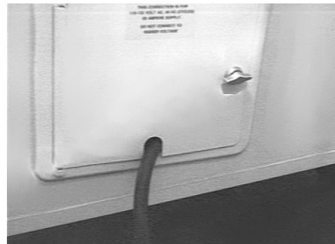
Shoreline shown routed through 'hatch' in compartment door on some models
