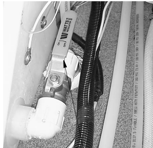
Water Tank Drain Valve (typical) Under Rear Bed or Couch
