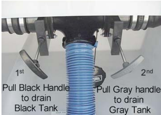
Holding Tank Dump Valves (Typical)
