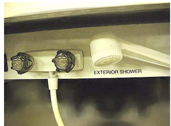
Exterior Shower/Wash Station (typical)
