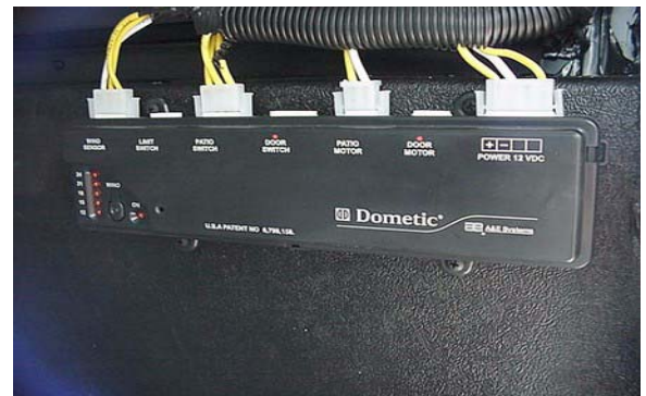
Awning Control Box (located in exterior compartment)
