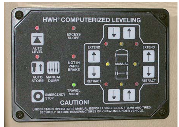
Leveling System Control Panel
