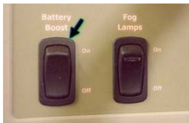
Battery Boost Switch
