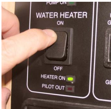
Gas Water Heater Switch (on Systems Monitor Panel)
