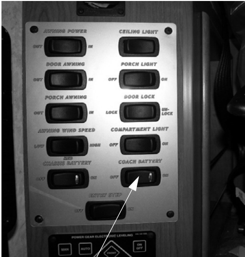
Auxiliary Battery Switch - Typical (Near Entrance Door)
