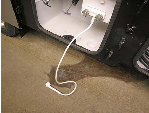
Using Exterior Shower to drain waterline (Typical View- appearance on your coach may differ)
