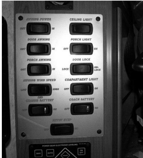
Awning Control Switches - Typical View (Located near entrance door)
