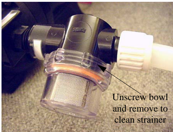
Water Pump Strainer (Located in water service center) -Typical View
