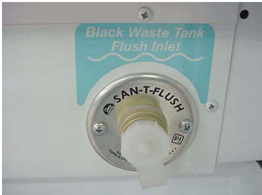
Water Tank Flush Inlet (typical)
