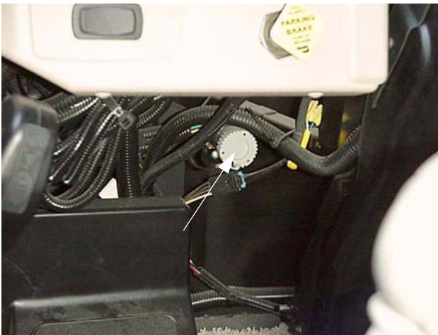
Diagnostic plug on steering column support beneath left side of dash -Typical View
