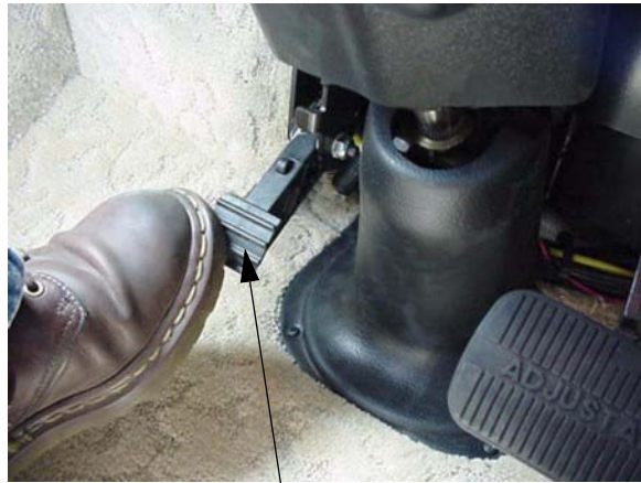
Press pedal to adjust steering wheel tilt or telescope
