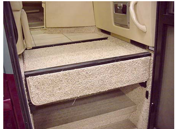
Step Cover shown in extended position (Typical)
