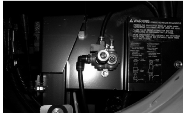
Quick Connect Air Coupler and Air Valve (located behind front hood)
