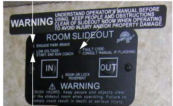
Low Voltage Indicator
