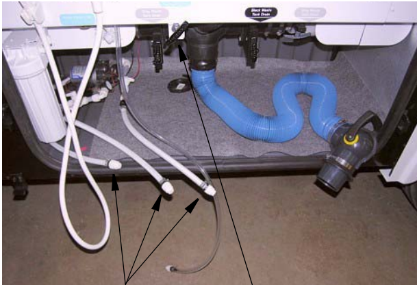
Waterline Drains (remove caps and turn valves to drain lines) Water Tank Drain Valve (pull T-handle to drain fresh water tank)
