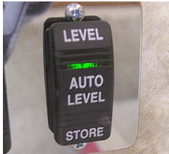
Auto Level Switch (Located inside entrance door)
