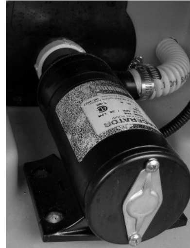
Waste Pump (Located beneath coach) -Typical View
