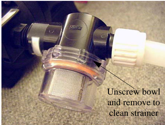
Water Pump Strainer -Typical View
