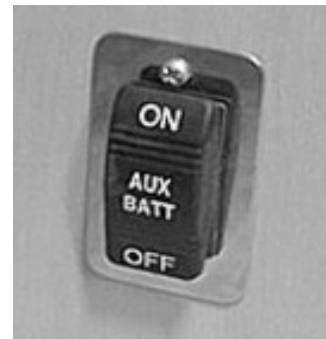
House/Coach Batt Disconnect Switch (Located near monitor panel) -Typical View
