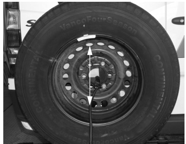
Incorrect Spare Tire Mounting Locations
