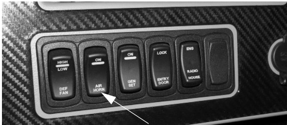
Air Horn Switch (Located on dash) -Typical View
