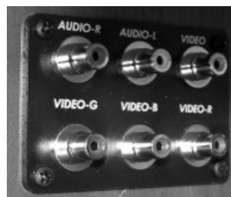
Audio Video Connection Plate -Typical View
