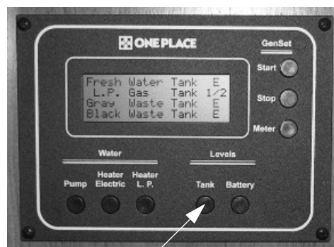
Tank Levels Switch
