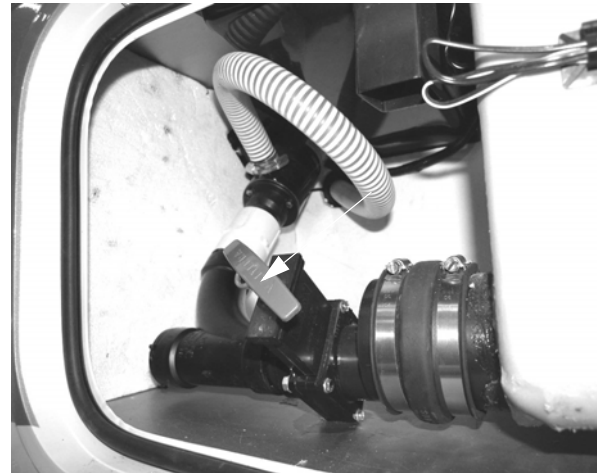
Gray Waste Tank Drain Valve (Located in driver side compartment behind rear wheel)
