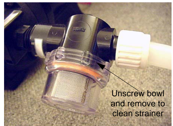
Water Pump Strainer -Typical View
