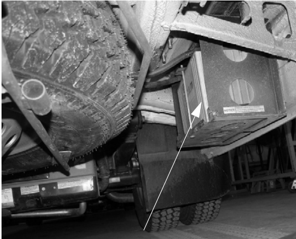
House Battery Access (Located behind rear passenger side tires) - Remove bolts from battery retainer to remove house battery
