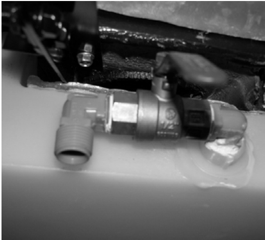
Water Tank Drain Valve (Located beneath running board, behind front passenger side door) -Typical installation shown
