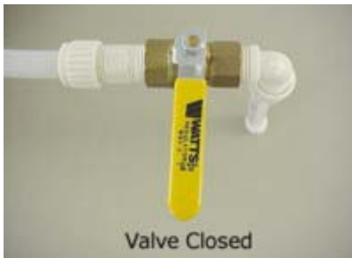
Water Tank Drain Valve (Located beneath running board, behind front passenger side door) -Typical installation shown
