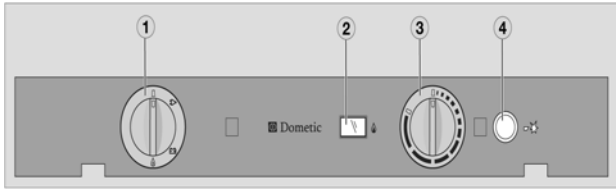
Refrigerator Operating Controls (Located inside refrigerator door)
