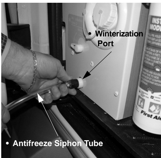
Antifreeze Siphon Tube/Winterization Port (Located near the sliding entrance door)
