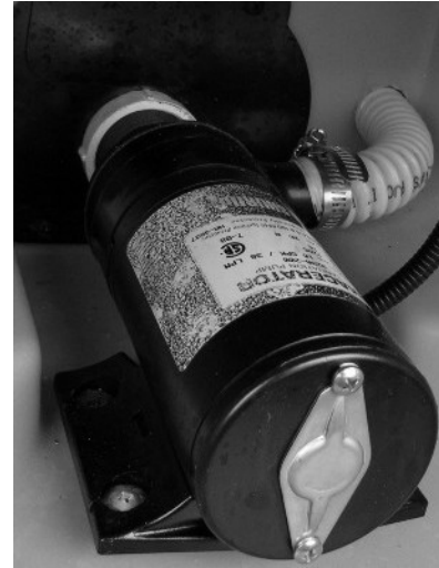
Waste Pump (Located beneath coach) -Typical View
