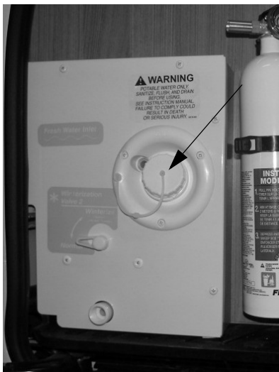
Water Tank Gravity Fill (Located near sliding entrance door) -Typical View
