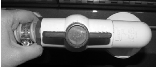
Sewage Drain Hose Valve
