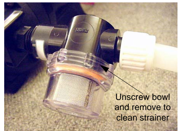
Water Pump Strainer -Typical View
