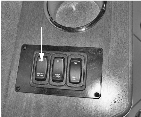
Power Door Locks - Entry Door (Located on passenger side trim panel) -Typical View
