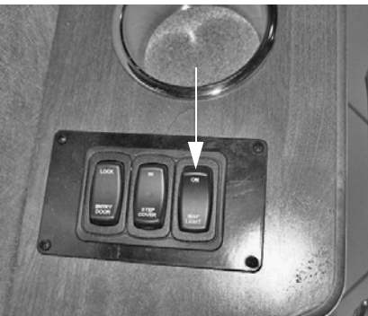
Passenger Map Light Switch (Located on passenger side trim panel) -Typical View
