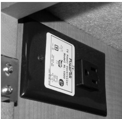
Front TV Ignition Switch Interlock –Typical View
