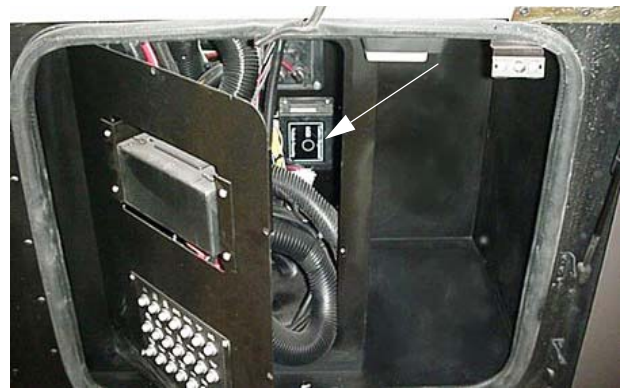
Keyless Entry Control Box (Located in 12-volt electrical compartment) -Typical View
