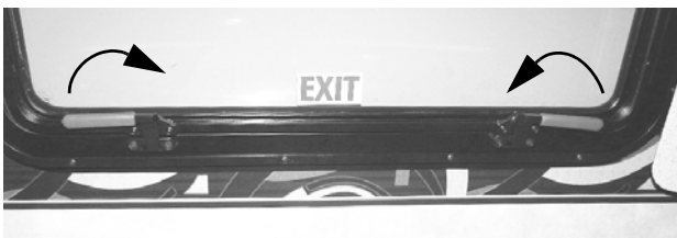
Escape Window (Lift latch handles upward to open)
