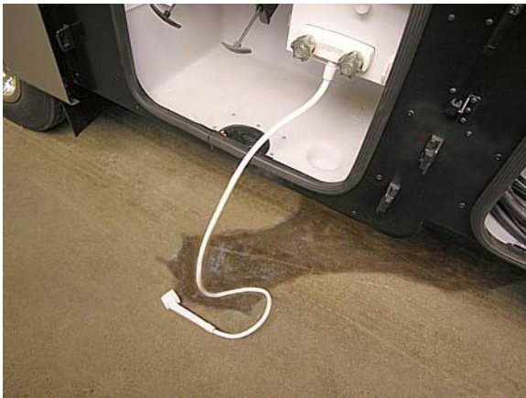
Using exterior shower to drain waterline -Typical View
