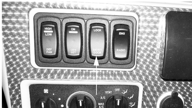
Power Door Locks - Entry Door (Located on dash) -Typical View
