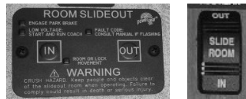
Slideout Switches (Your coach may have one or more of these switches depending on model, options, and available equipment) -Typical View
