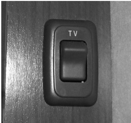
12-Volt TV Master Power Switch (Located in overhead cabinet or on a wall near the TV) -Typical installation shown
