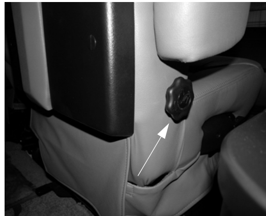
Lumbar Adjustment Dial (Located on the side of driver and passenger seats)
